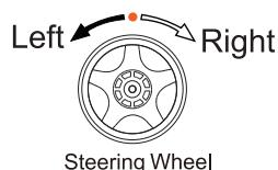
If the steering angle is too small, adjust the D/R counter-clockwise.
