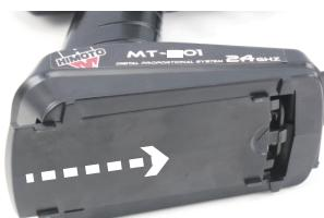
Incorrect battery insertion could damage the transmitter. This 2.4Ghz transmitter has an internal Antenna.
