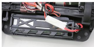
You need to insert the battery pack in the open section for the battery. Use the chassis cut-out for corner wiring if needed. Use the straps provided to secure the battery in place.
