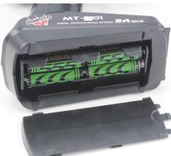
Open the battery holding tray. Insert 4 AA batteries into the marked spaces. Please note the correct direction of the batteries.
