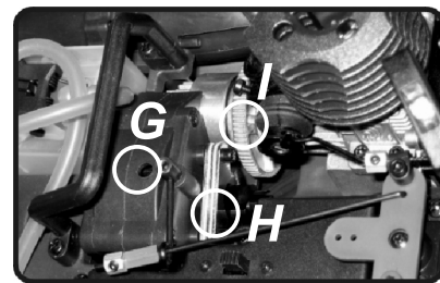
(G) High quality 2-way gear built in compact gear box free from friction (H) High performance brake discs (I) 13.8g lightweight flywheel performs quick engine response.
