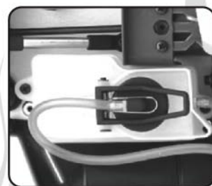
Extra large fuel tank with spring load fill cover is perfect for re-fueling.
