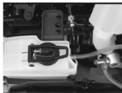
Leak Proof Fuel Tank With Overflow Pipe
