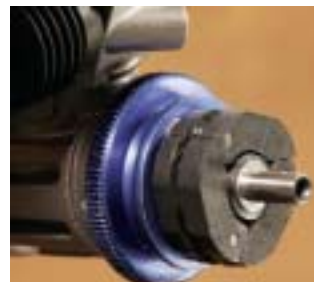
A three-shoe composite clutch comes standard on the Torpeda.
