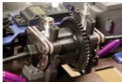
The Torpeda's center diff features a steel spur gear and single-disc front and rear brakes with brake disk guides.
