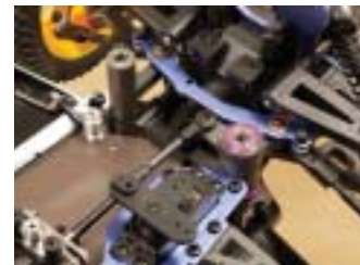
Steering on the Torpeda is standard 1/8-scale buggy fare. A high-torque steering servo's output is transferred through a cam-style servo saver to the front wheels. Notice the shock-absorbing spring located on the lower left hinge pin.
