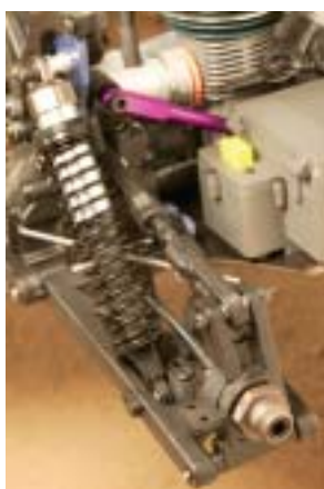
The rear suspension of the Rancho is comprised of a lower composite arm and an adjustable upper control link.
