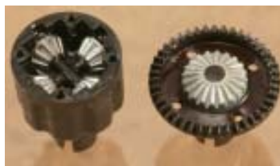
The Rancho features six gear differentials in both front and rear for durability.
