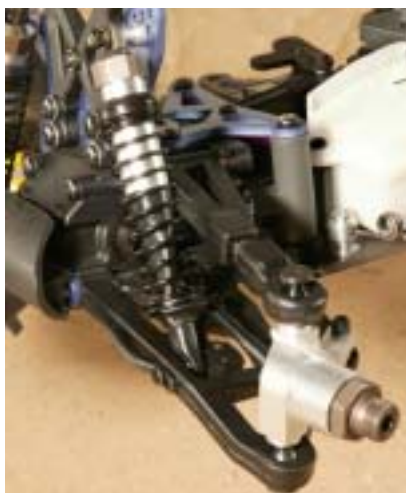
Coil-over, oil-filled shocks and aluminum steering knuckles contribute to the good handling of the Rancho.
