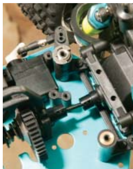
Bushing-supported bellcranks handle the steering duties with a servo saver built into the main crank.
