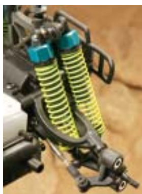
Static suspension components are found in the rear. Notice the standard hex pins on the axles. This allows the use of many different wheels down the road.
