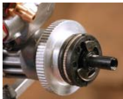
A two-shoe racing style clutch is used to get the truck moving; the aluminum flywheel is a nice touch.
