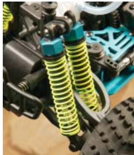
Two shocks per wheel is the name of the game for the Mini Cobra. These large, oil-filled shocks soak up all the bumps along the way.
