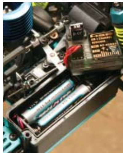
The radio box takes up much of the left side of the chassis and houses everything but the servos. To power the truck, Himoto used a super small four-cell AAA receiver pack.
