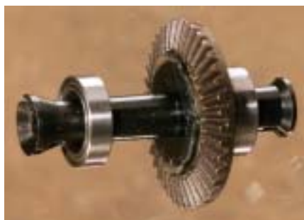
Both front and rear differentials on the Mini Cobra are fully supported by ball bearings to ensure smooth operation.
